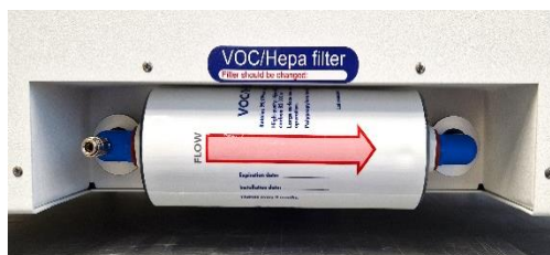
Figura 12.3 Filtru COV/HEPA corect instalat
